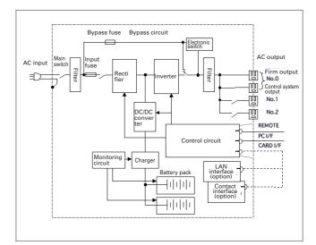
Fig. 4 "SANUPS A11G-Ni" circuit system diagram
