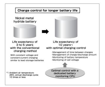
Fig. 3 Elements of optimal charging control.
